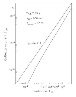
Figure 2. Sensitivity of the reflex sensors' detector
