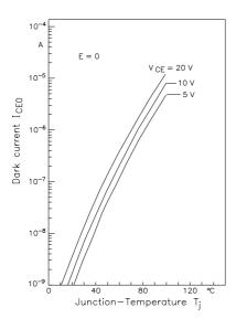
Figure 10. Temperature-dependence of the collector dark current
