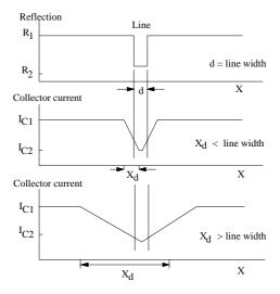
Figure 8. Reflection of a line of width d and corresponding curve of the collector current I<sub>c</sub>
