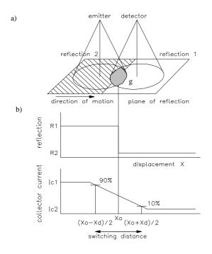
Figure 7. Abrupt reflection change with associated I<sub>c</sub> curve
