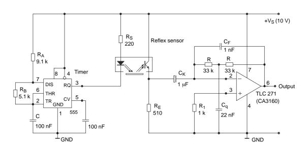
Timer dimensions:  $\begin{array}{ccc} t_p \text{ (pulse width)} = 0.8 \text{ RC} = 400 \text{ }\mu\text{s} \\ T \text{ (period)} &= 0.8 \text{ }(R_A + R_B) \text{ } \times \text{ } C = 1 \text{ ms} \\ \\ \text{Active filter}: & C = \sqrt{C_f \times C_q} & Q = \sqrt{\frac{C_q}{C_f}} \\ \\ f_o = 1/(6.28 \text{ } \times \text{ } C \times \text{ } R) & V_{uo} = \frac{2 \text{ } R}{R_E} \times Q^2 \\ \end{array}$
