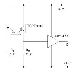
Figure 11. Reflex sensor - basic circuit
