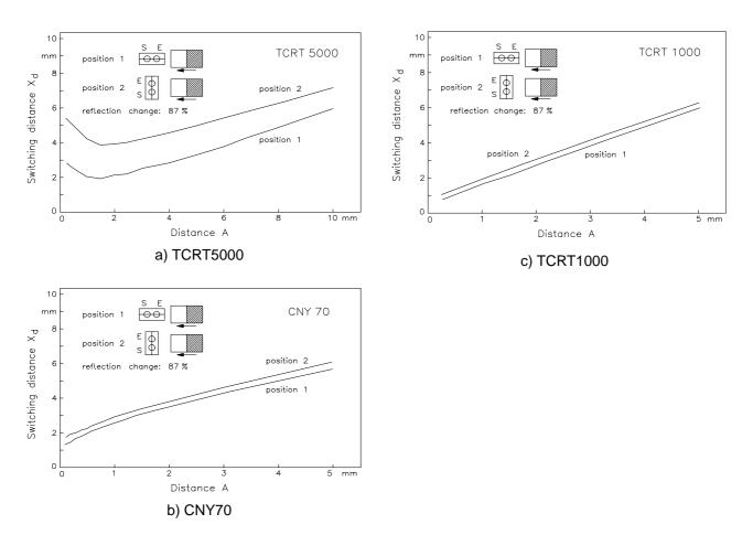
Figure 9. The switching distance as a function of the distance A for the reflex sensors TCRT5000, CNY70 and TCRT1000
