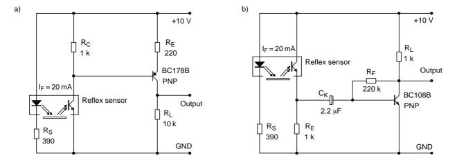
Figure 13. Circuits with transistor amplifier
