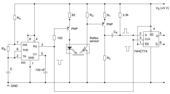
Figure 18. Pulse circuit with buffer storage
