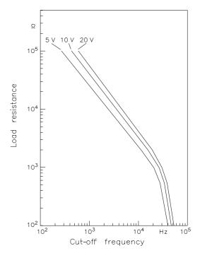
Figure 5. Cut-off frequency, f<sub>c</sub>
