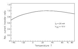
Figure 4. Change of the coupling factor, k, with temperature, T
