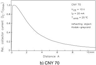
Figure 6. Working diagram of reflex sensors TCRT5000, CNY70 and TCRT1000
